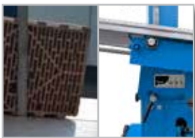
Inclined cut on bricks with empty cavities
